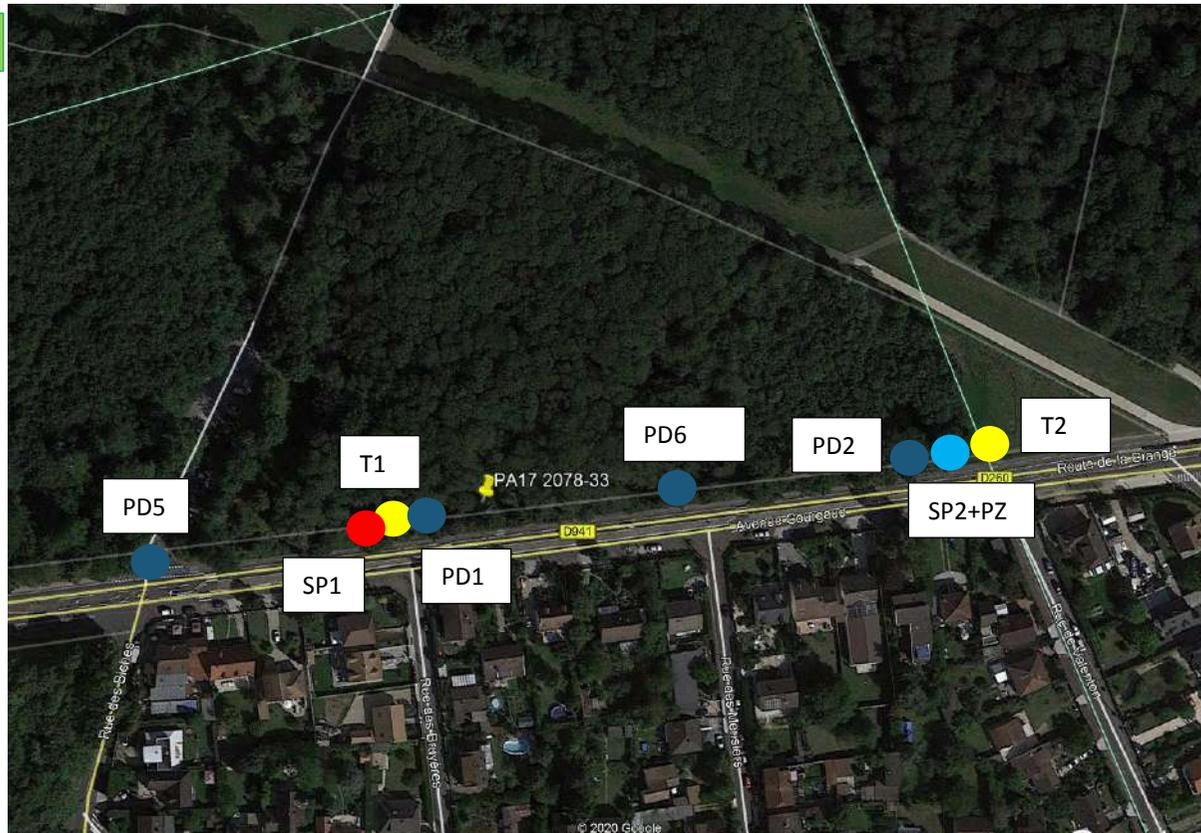
SCHEMA D'IMPLANTATION DES SONDAGES IN-SITU
