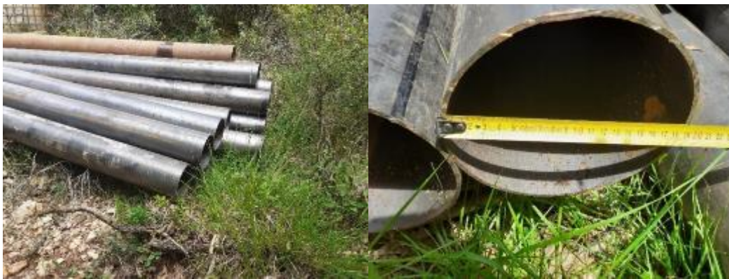
Figure 12 : Tubage acier diam. 193 mm
